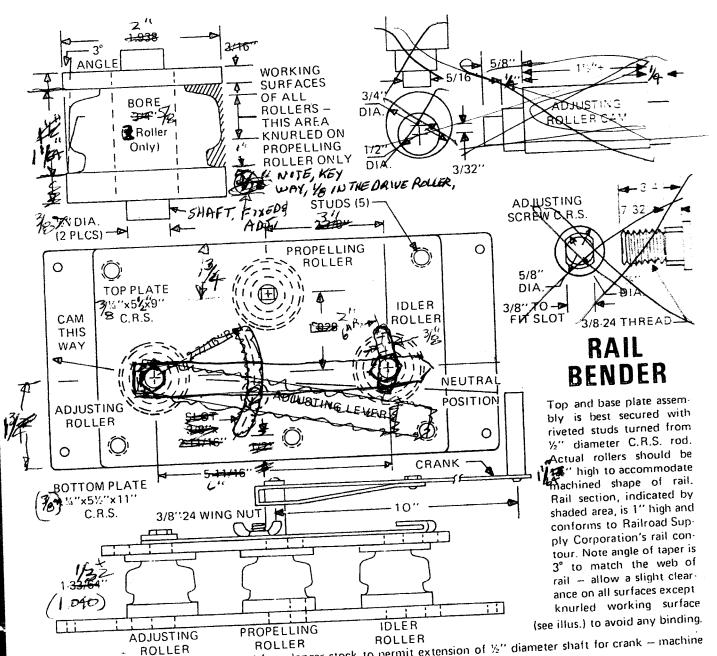
Propelling Roller must be fabricated from longer stock to permit extension of ½" diameter shaft for crank - machine
